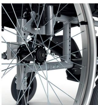
Different adjustment possibilities for the seat height and seat depth
